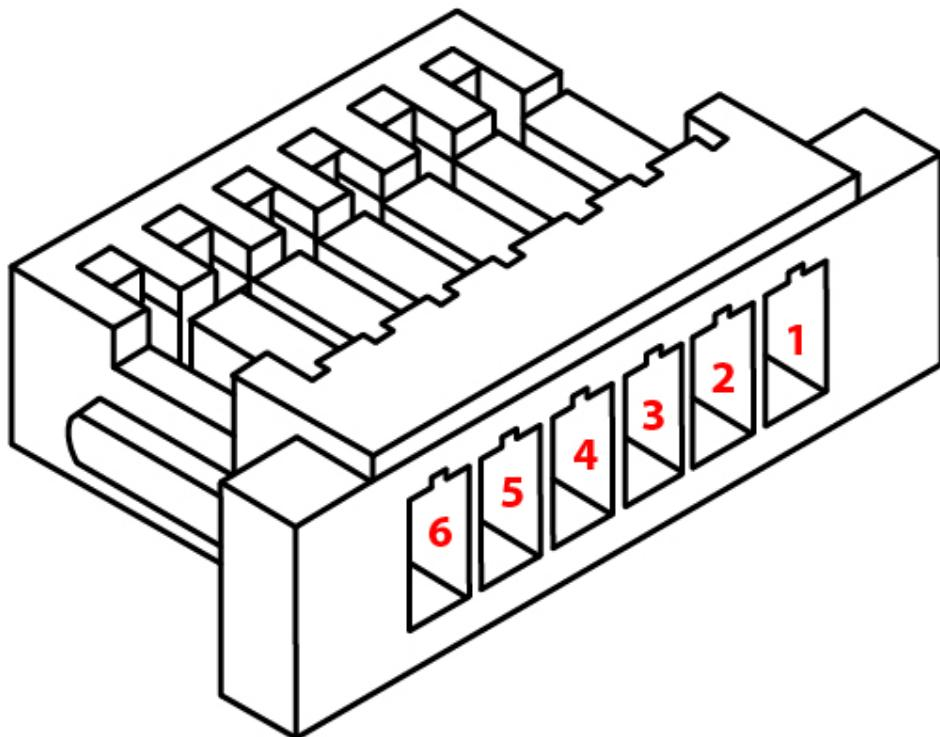
**J3 (RS232) pinout of female connector**
