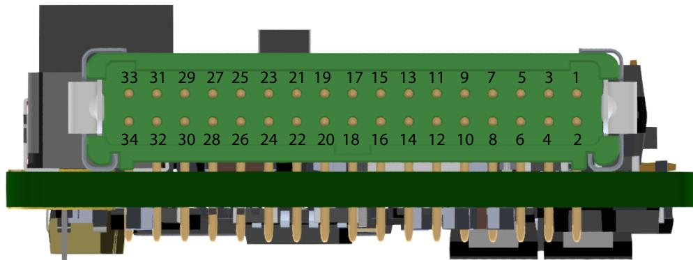
**MEX connector pinout**
