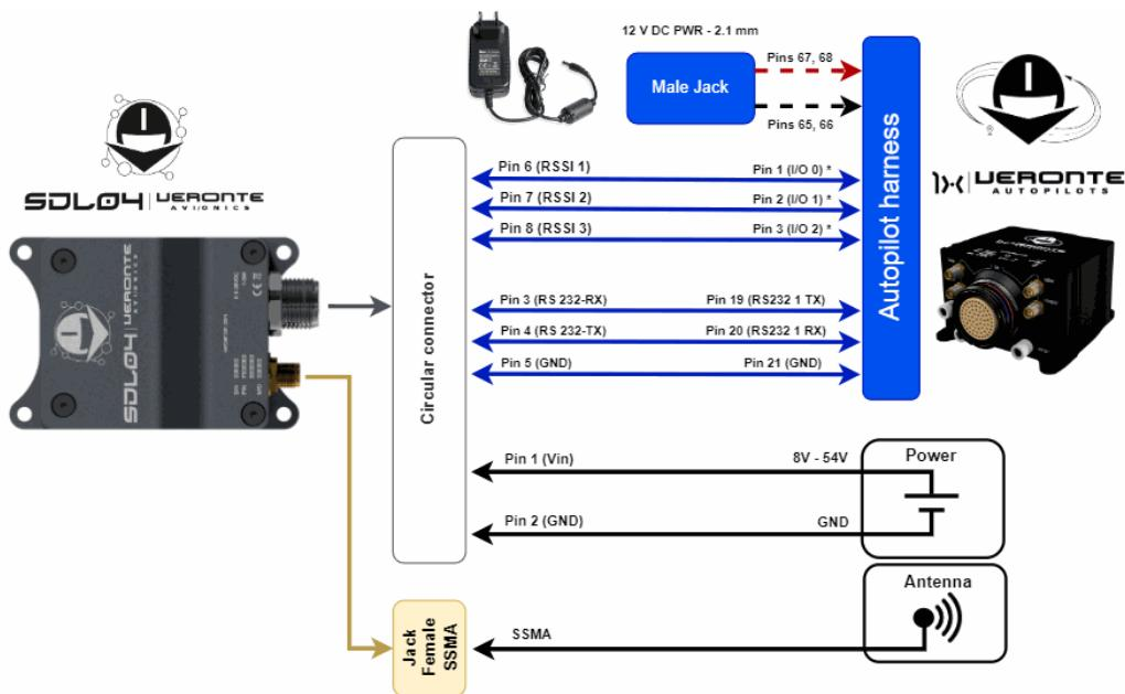
\* Those signals are configurable I/Os. This is only an example, users can choose from the following 1x pins to connect: 1, 2, 3, 4, 5, 6, 7 or 8
