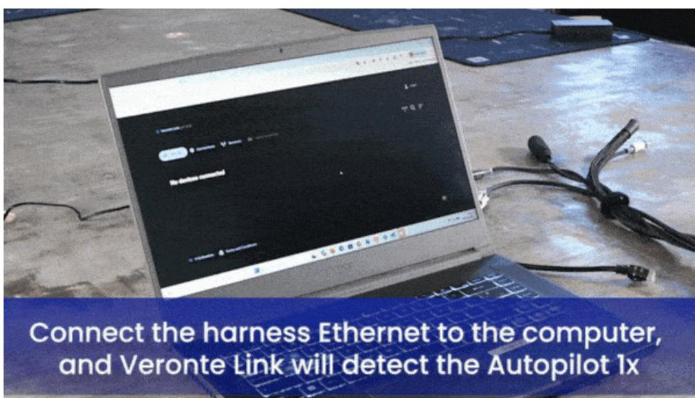
**Connect the harness Ethernet to the computer, and Veronte Link will detect the Autopilot 1x**
