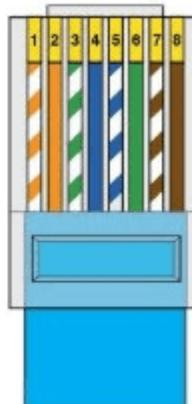
**RJ45 pinout T-568B**
