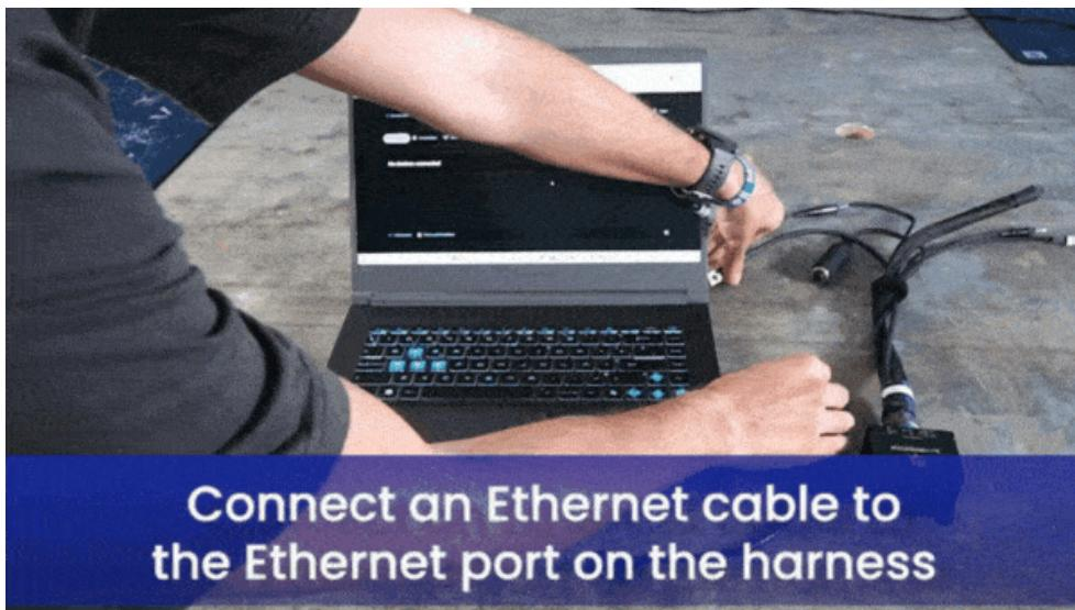
**Connect an Ethernet cable to the Ethernet port on the harness**
