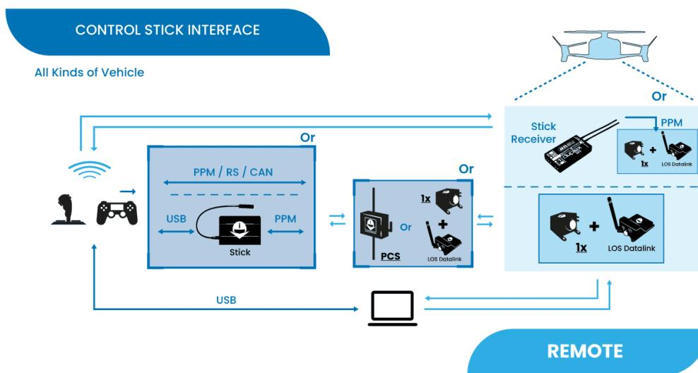
Although the most common way of control is to directly connect a **stick** via **PPM**, **RS** or **CAN** to a control station (**PCS/1x + LOS Datalink**) which then communicates with the onboard autopilot,
